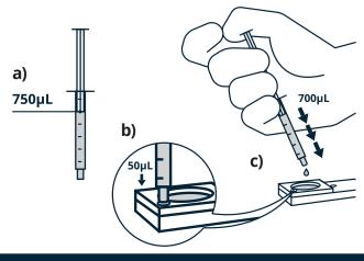
**4** a) Draw 750µL of media. b) Prime outlet channel. c) Cover membrane surface.
